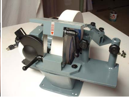
Fig. 10 Completed vertical mount installation
