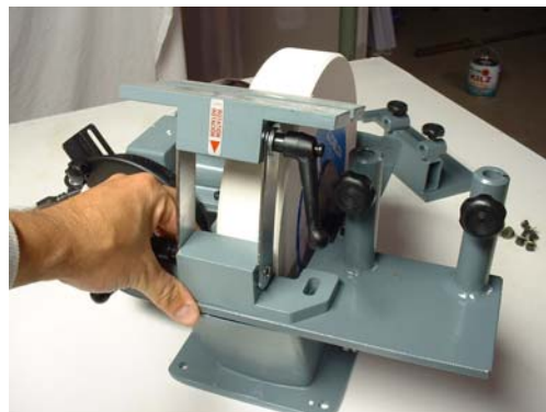
Fig 7. Alignment of base with machine. Fig 8. Alignment of toolrest and mount bases
