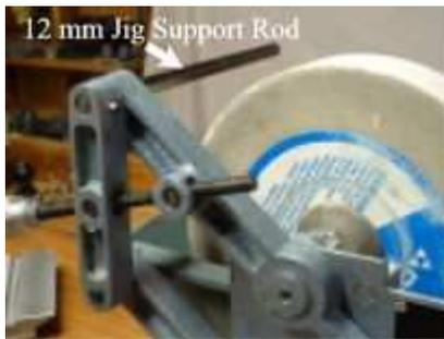
**Step 1:** Turn off the grinder! Remove the flat rest support casting by loosening the socket cap screws that secure it to the 12 mm support rod.
