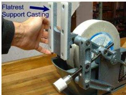
**Step 3:** Adjust rod height using the leadscrew adjustment knob to the desired position for your jig.
