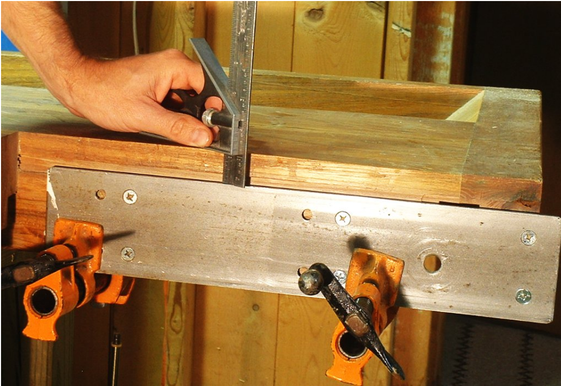
Figure 34: Ensuring that the steel plate is parallel with the bench top
