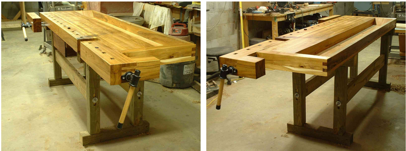
Figure 1: A finished workbench; black locust top on a pressure treated lumber trestle
